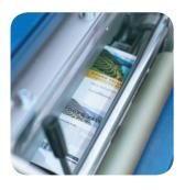
2. MEMJET VERSAPASS SINGLE PASS PRINTHEAD Prints either 29.5' or 59' per minute
